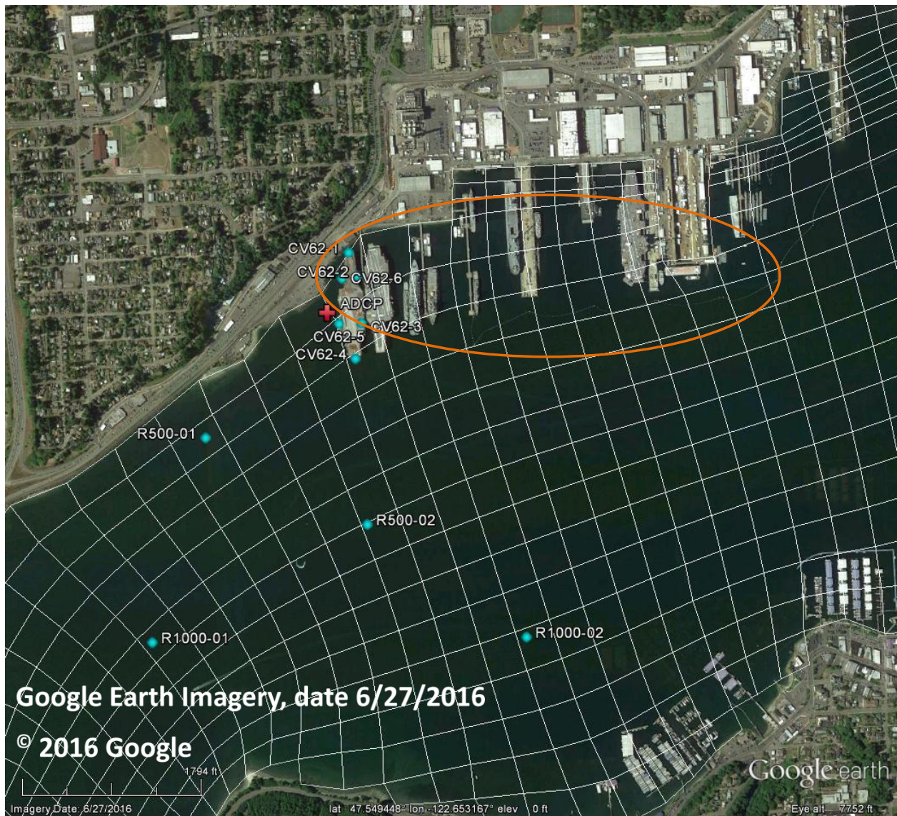
Figure 8. Location of water quality monitoring stations directly adjacent to the ex-INDEPENDENCE (CV62-1 to CV62-6), reference stations (R500-01, R500-02, R1000-01, and R1000-02) outside of the area of influence (orange oval), location of ADCP (red cross), and overlay of CH3D model grid (white rectangles).
