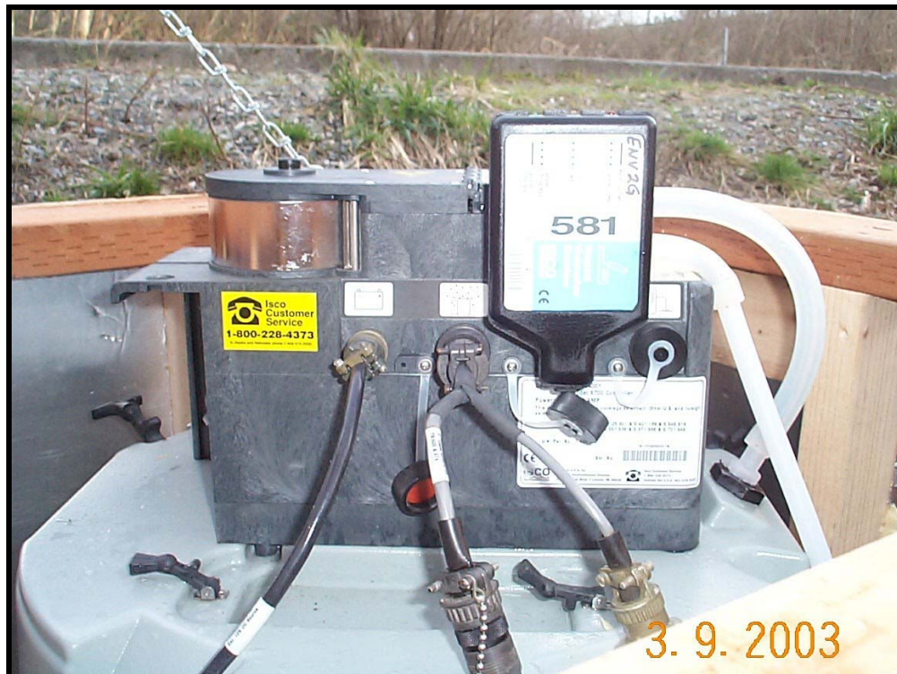
Downloading data from Isco using RTD – post sampling.
