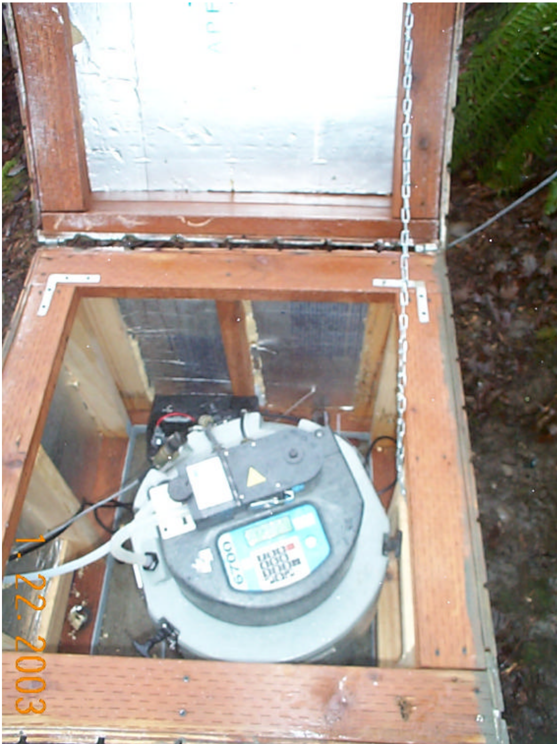
Inside of Sampling "Box" Depicting Isco, Tubing, Cables, and Battery
