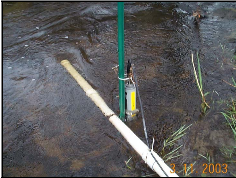
11 March – CC – Low water prior to storm. Note leaves caught up in the “top” of the Sonde – high water mark from Storm #6a.
