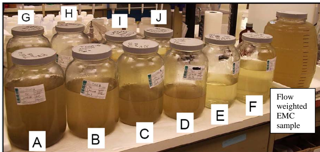
Figure 4 Time-Paced Interval Jars (A thru J) and the Flow Weighted Composite (EMC sample) from Outfall LMK038 Manchester, Each Jar Represents a 3-hour Interval of the Storm
