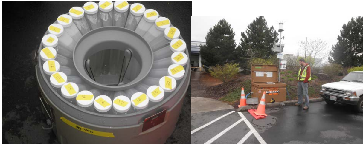
Figure 3-2 Composite sampler ring with 1-hr composite wedge bottles labeled 1 through 24. On the left the field sampling box with the rain gauge and telemetry system.
