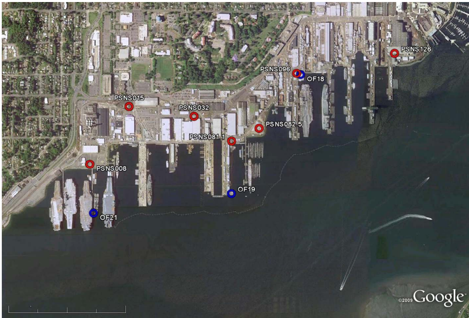
Figure 3. Industrial outfall discharge locations (blue circles) and stormwater outfall sampling locations (red circles) to be monitored during WY2011 (TAI 2009, 2010).
