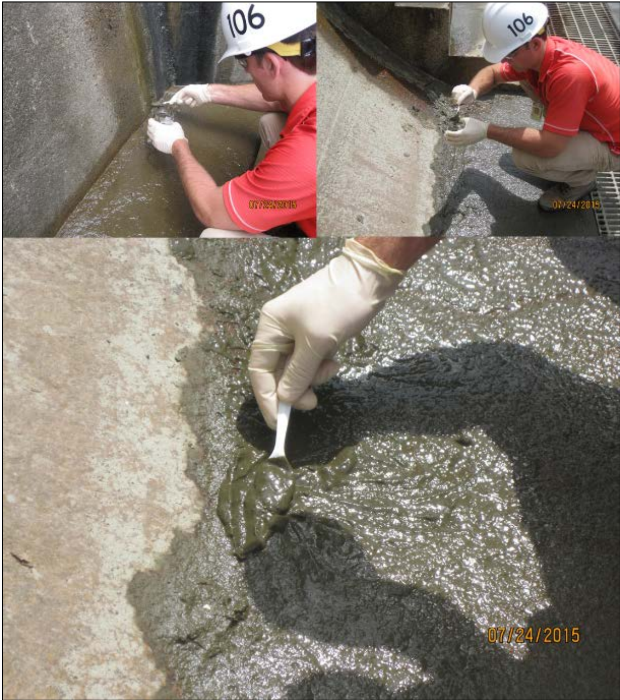
Figure 33. Example of collecting silt samples from dry dock floor after dewatering. DISTRIBUTION STATEMENT A. Approved for public release; distribution is unlimited.
