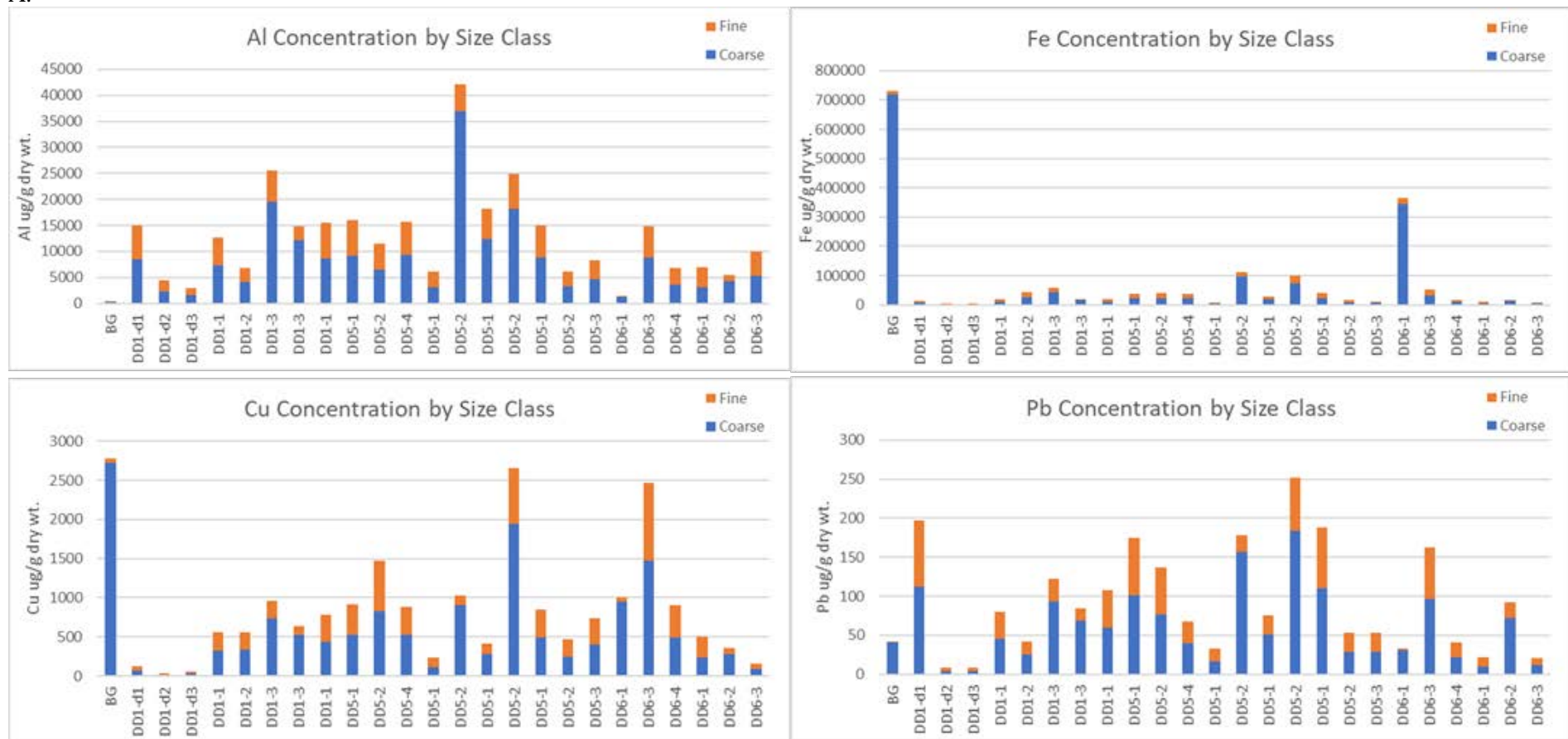
Figure 62. The concentrations of metals measured in coarse and fine fractions of BG and dry dock silt samples collected in 2012-2014 for Al, Fe, Cu, and Pb (A), and Zn, Hg, Ni, and Cr (B).
