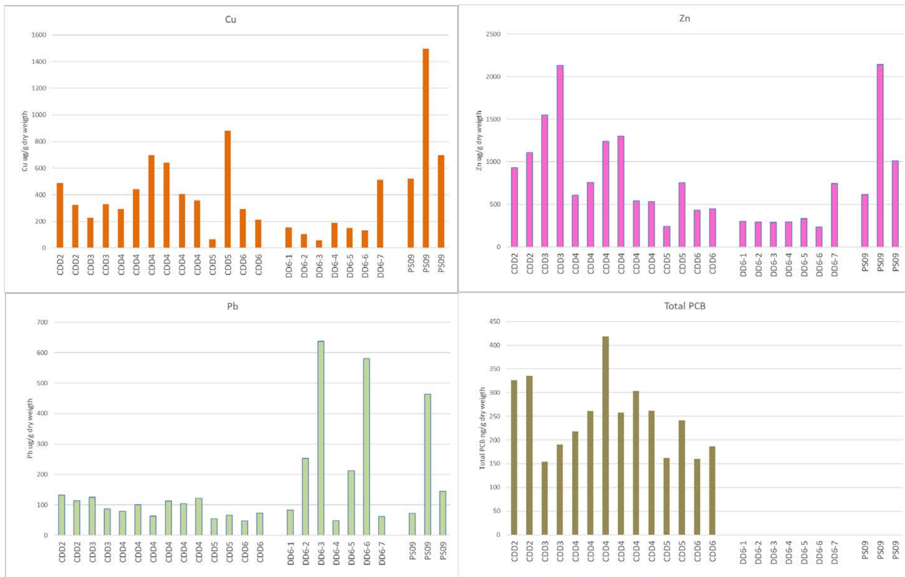
Figure 61. Concentrations of Cu, Pb, Zn, and Total PCB measured in caisson and dry dock silt samples collected in 2009-2010.
